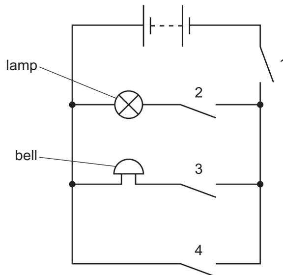
Which switches must be closed for the lamp to light and the bell to ring?
