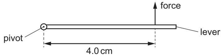
The force is exerted 4.0 cm from the pivot. The moment of the force about the pivot is 8.0 N cm.
